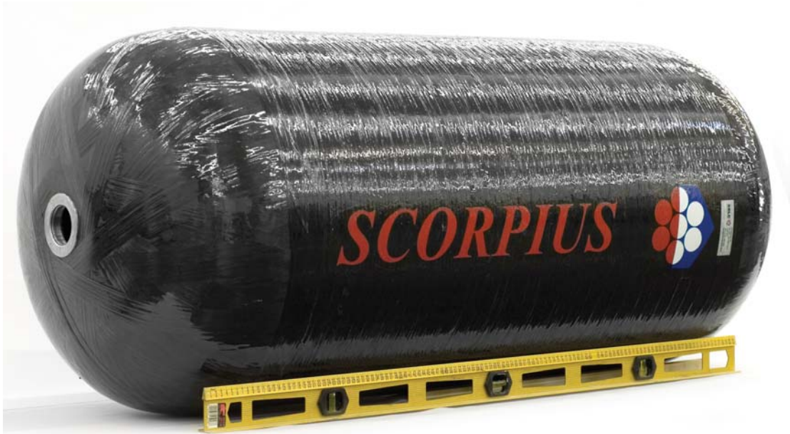
A 25" diameter high-pressure tank, 60" long, all composite liner-less for liquid cryogenics.
